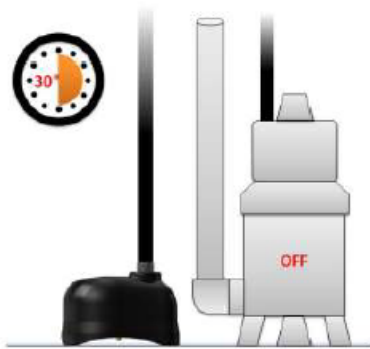
Crab turns OFF the pump 30 seconds after the 2 sensors don't detect the water anymore to let the pump empty the system
